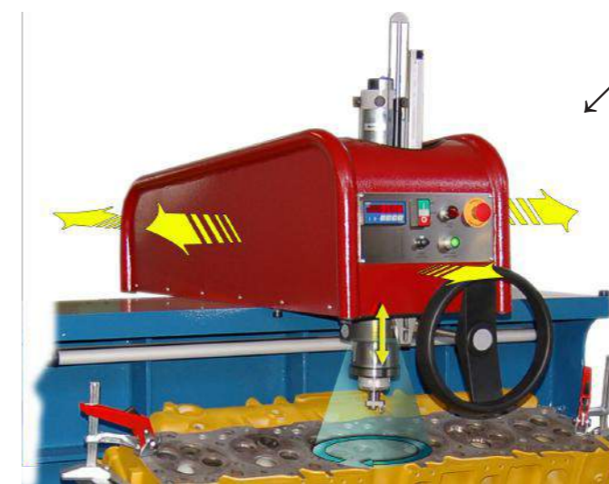
Spindle head and cylinder heads support move on an air cushion in all directions, by an electromagnetic locking system
